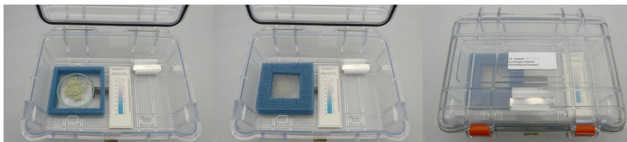
Figures 7 – 9: Layout of control setup. H 2 S powder is covered over with a piece of fine woven nylon gauze. Silver coupon is placed in a piece of recessed PE foam adhered to the lid on the inside of the dry box
