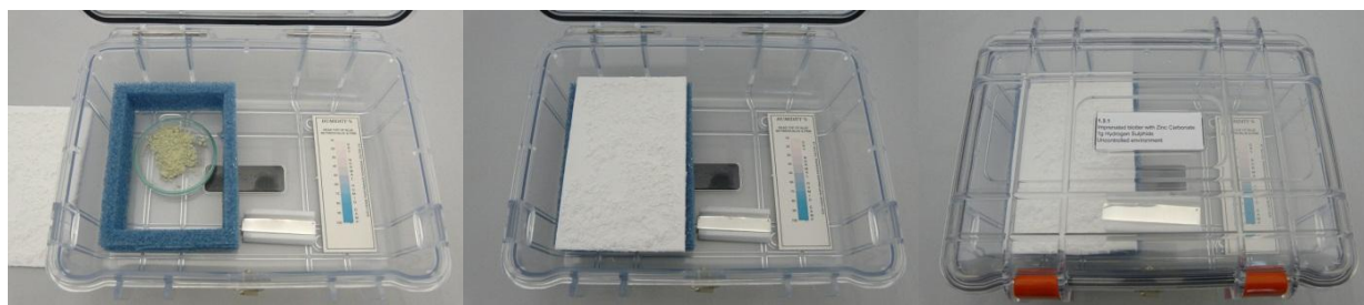
Figures 10 - 12: Layout of self-made H 2 S sorbent with zinc carbonate. The scavenger is placed directly on top of the pollutant H 2 S
