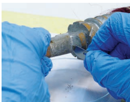
Figure 2. Removing a small sample from the surface of a suspected object for testing
