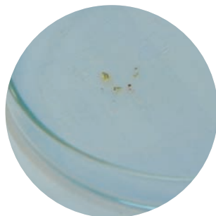
Figure 5. If there is no presence of mercury, no blue violet complex will appear
