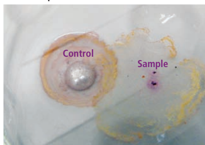
Figure 4. Sample shows the formation of a blue violet complex, which indicates the presence of mercury in the object; there is no such complex in Control
