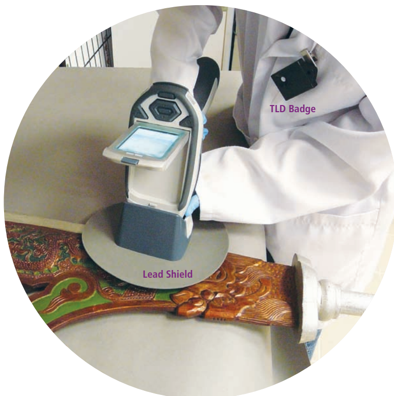
Figure 6. A user wearing TLD Badge while using the Thermo Scientific Niton XL3t GOLDD XRF Analyser that comes attached with a lead shield
