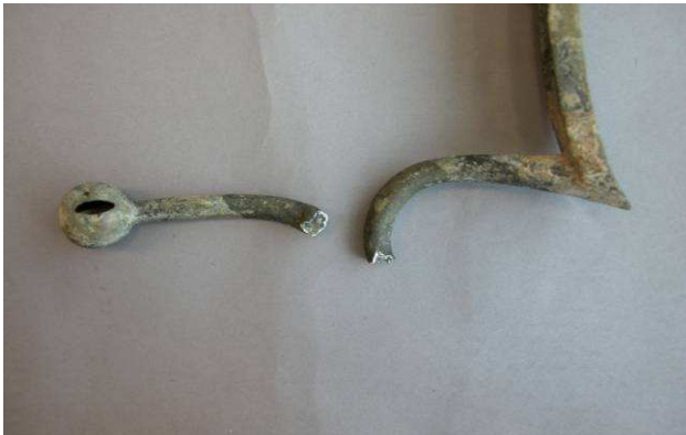
← The broken arched shaft.
