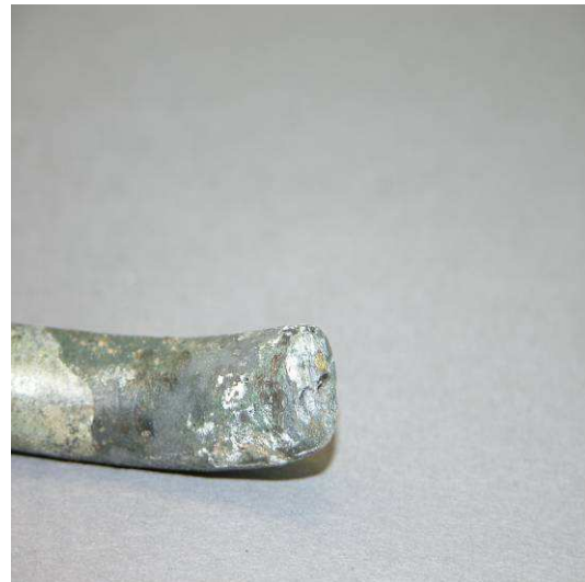
↑ A view of a broken brass dowel.
